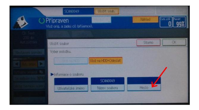
The password can be up to 8 characters long and it must only be numeric (0-9). After entering the password on the copier's numeric keypad, the machine will prompt you to confirm the password, and then press "**OK**" twice.
